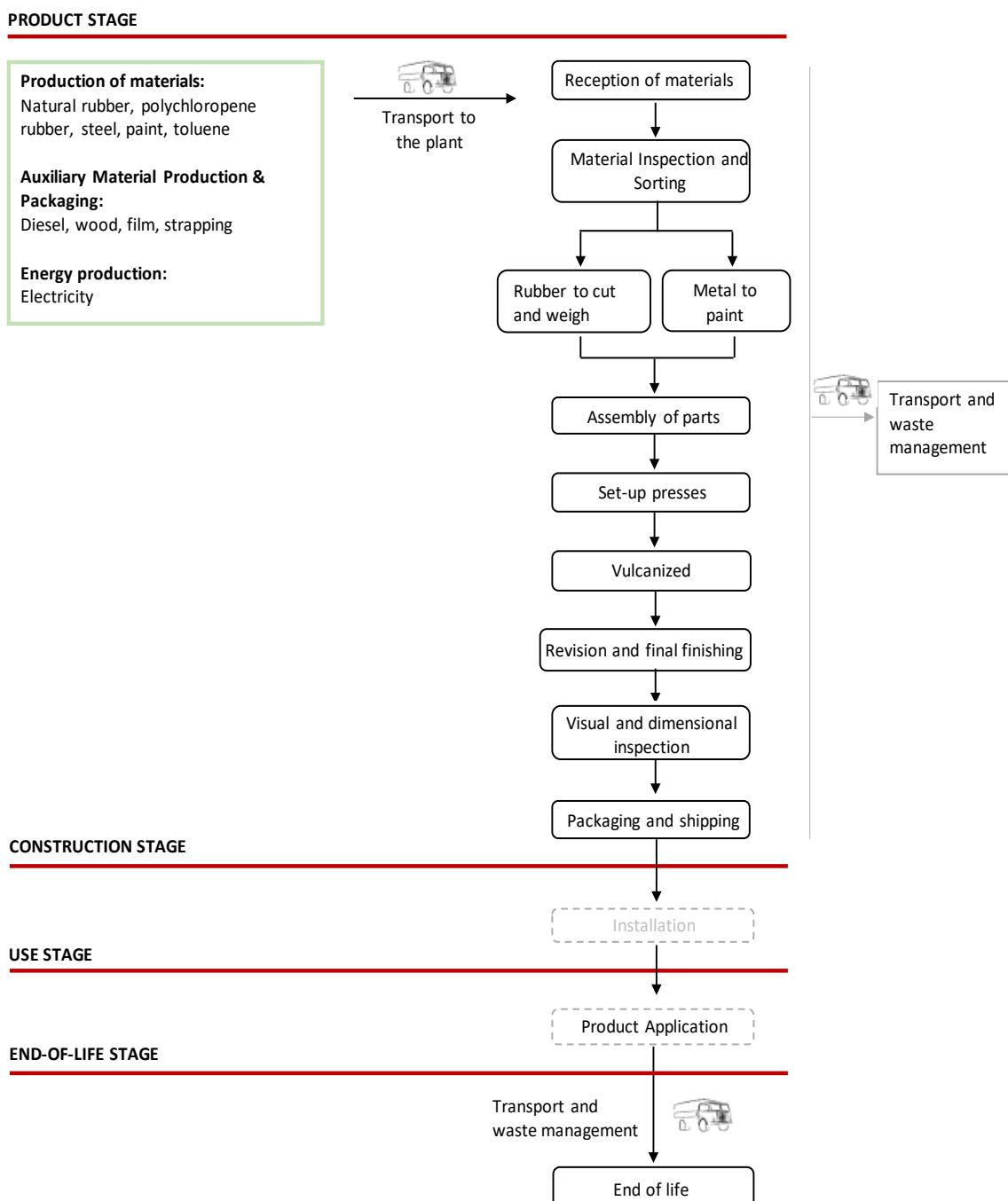
The manufacturing process begins with the supply of rubber laminate at the manufacturer's premises. After receiving and verifying the goods at CACESA's facilities, the manufacturing processes of the supports are carried out.
