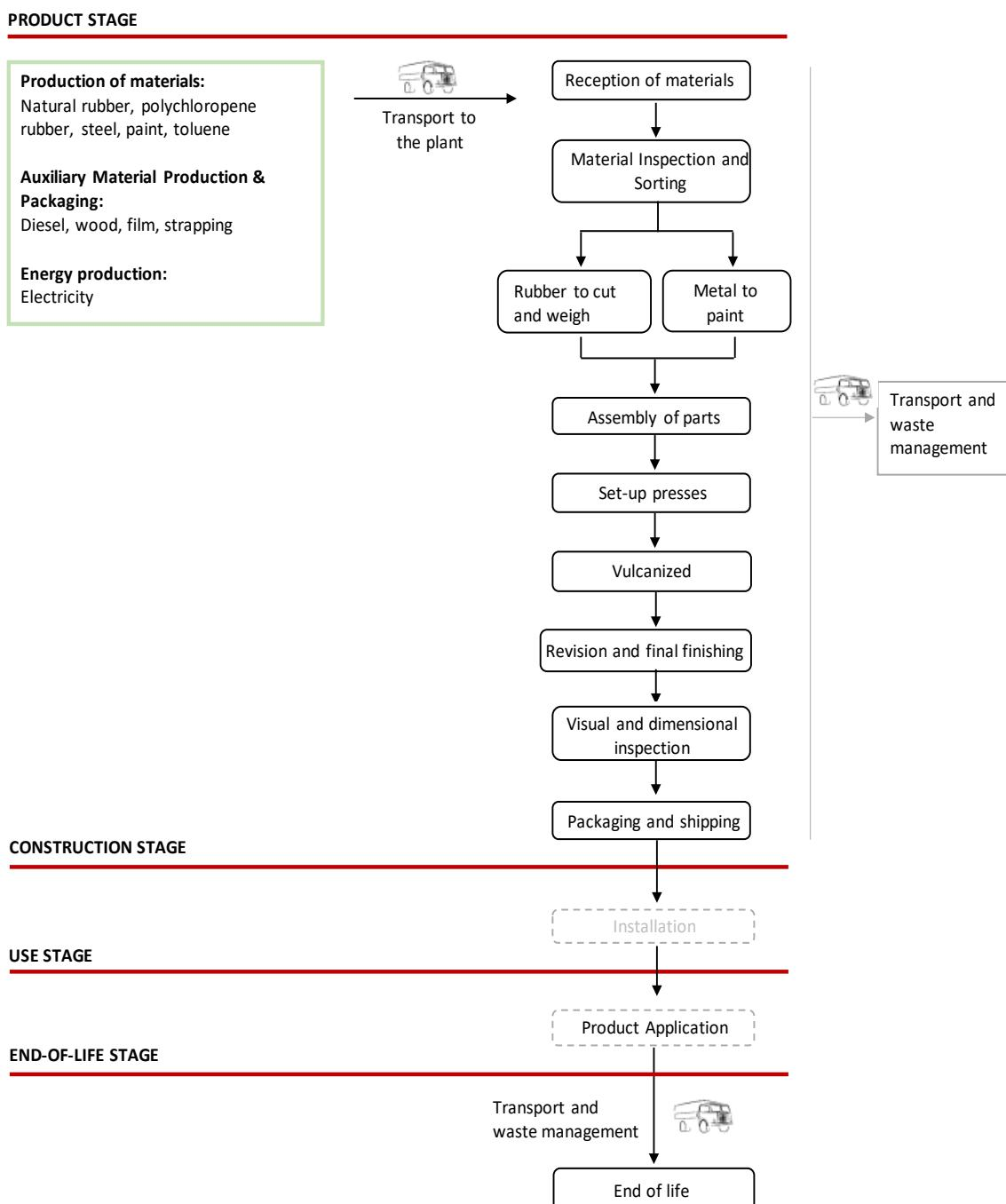
The manufacturing process begins with the supply of rubber laminate at the manufacturer's premises. After receiving and verifying the goods at CACESA's facilities, the manufacturing processes of the bearings are carried out.
