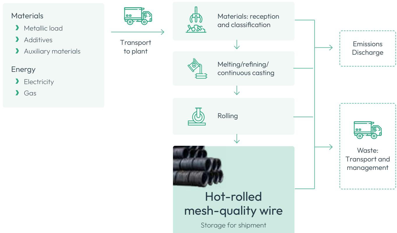
The factory produces steel using the electric arc furnace route. The steelworks mainly melt scrap metal, adjusting the chemical composition to obtain the required steel specifications. The resulting material is solidified into billets of different sections and lengths, which constitute the intermediate product used as raw material in the hot rolling process.
