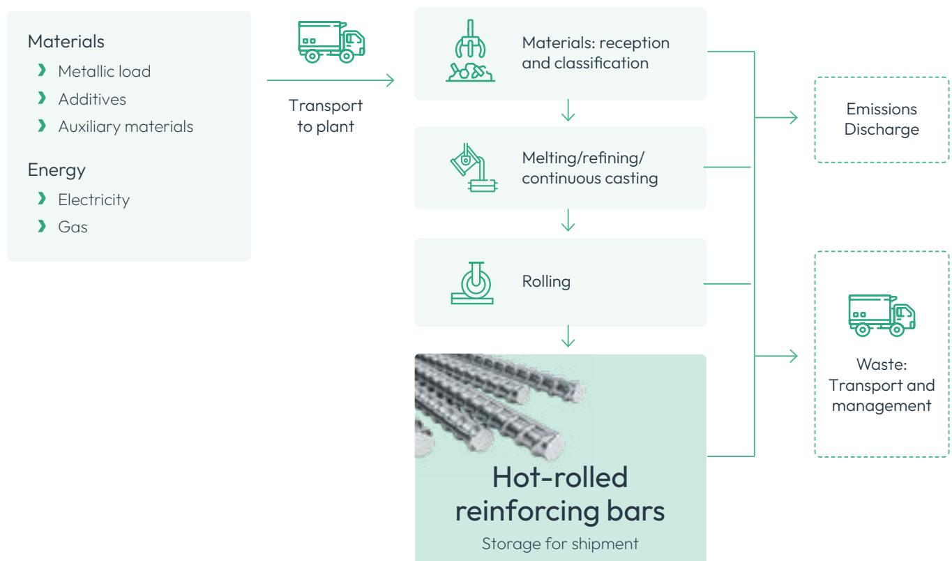
The Megasa Group's factories produce steel using the electric arc furnace route. The steelworks mainly melt scrap metal, adjusting the chemical composition to obtain the required steel specifications. The resulting material is solidified into billets of different sections and lengths, which constitute the intermediate product used as raw material in the hot rolling process.
