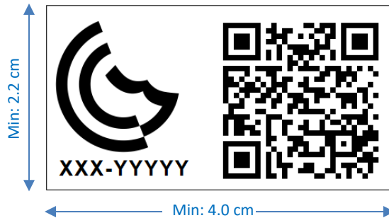
Fig. 2: Minimum dimensions of the GCTS for Certificates
